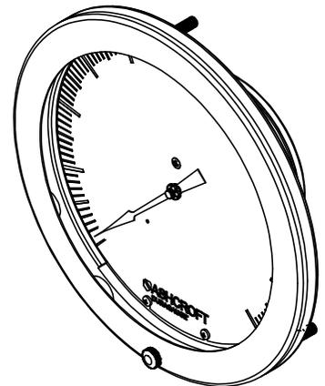
Note: 3 Mounting studs threaded equally spaced on a 9.625" [244] Bolt Circle.
